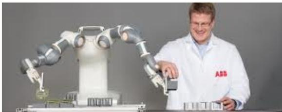
Figure 1: ABB FRIDA robot acting as a robotic assistant
