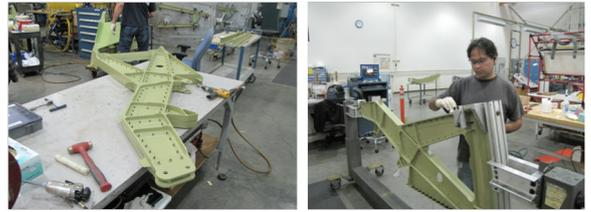
Figure 2: Spar assembly is a manual process that could be improved by a robotic assistant
